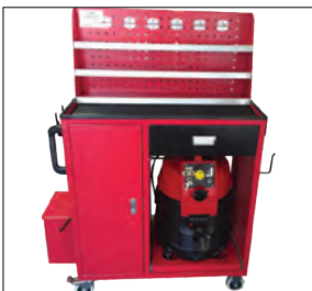
Mobile Workstation with EP Vac & 2x Air/Dust Hoses
